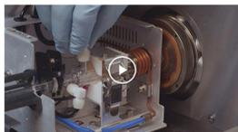
Eliminate plasma ignition problems and maintain optimal performance. Learn how to inspect the torch, bonnet, shield plate, and RF coil. We'll also show you how to clean the torch.
