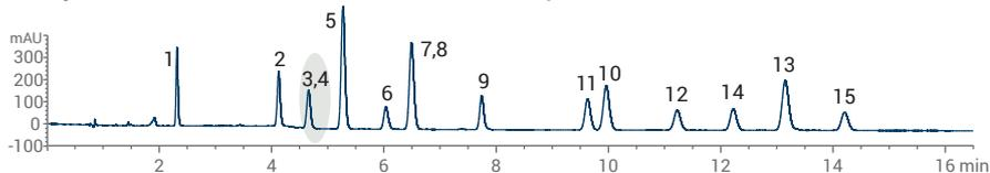
**InfinityLab Poroshell 120 Phenyl-Hexyl, 4.6 x 150 mm, 2.7 μm**
