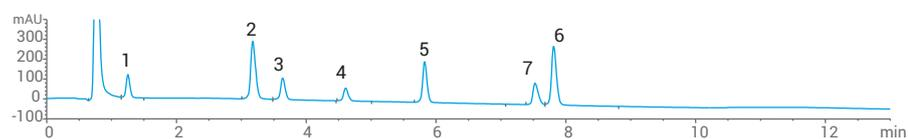
InfinityLab Poroshell 120 Phenyl-Hexyl, 2.1 x 100 mm, 2.7 μm
