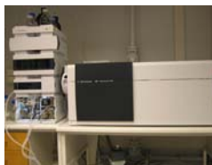
Figure 2. An Agilent 1290 Infinity LC system was coupled to an Agilent 6460 (Jet Stream) Triple Quadrupole instrument.
