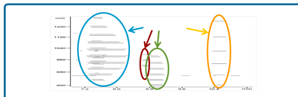
Figure 4. The peaks corresponding to different charge states of the same protein elute at the same time in the LC/MS run. Each oval corresponds to a unique coelution groups, each of which produces one or more protein compounds using algebraic deconvolution.
