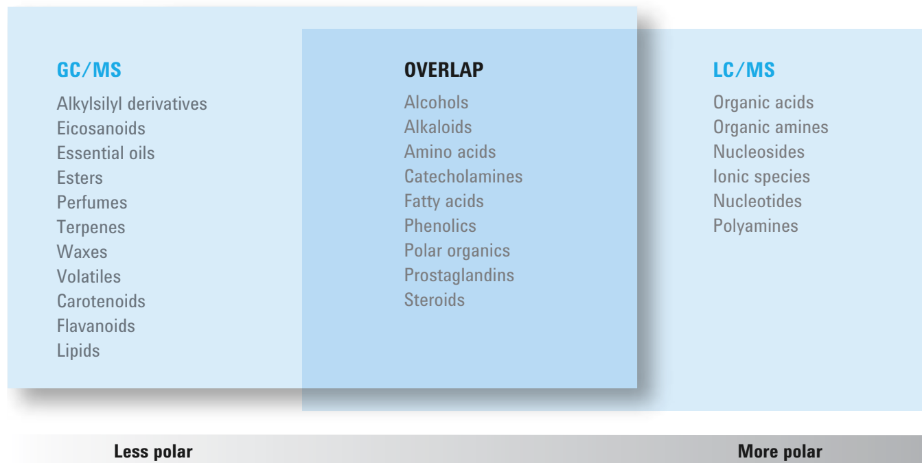
Chemical classes suitable for GC/MS versus LC/MS
