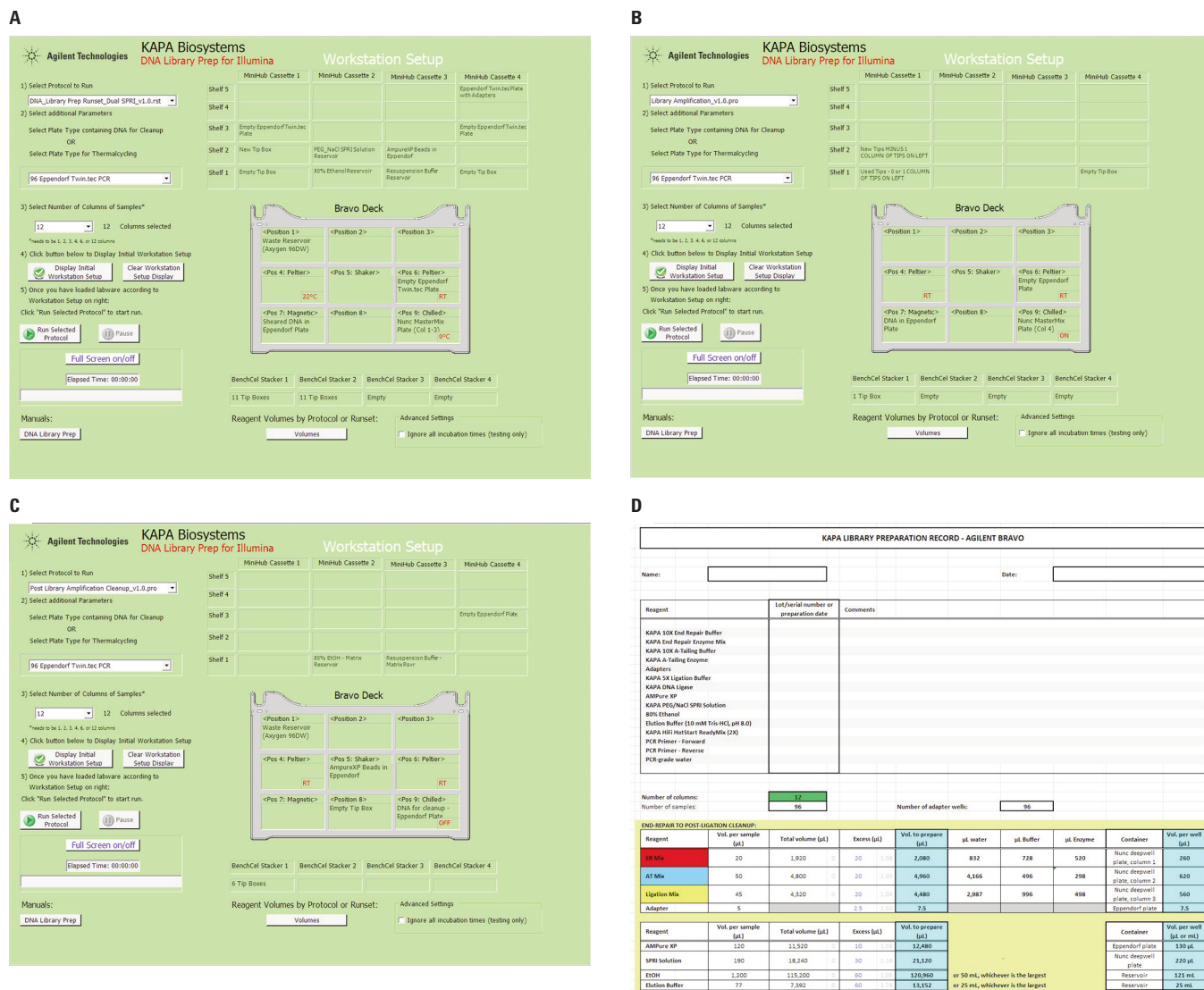
Figure 4. VWorks Forms and a Microsoft Excel workbook for the KAPA HTP Library Preparation method. A) End Repair to Post-ligation Cleanup Form, B) Library Amplification Setup Form, C) Post-amplification Cleanup Form, D) Microsoft Excel workbook. Each run is configured by selecting the number of plate sample columns (1, 2, 3, 4, 6, or 12 columns, and 8, 16, 24, 32, 48, or 96 samples), after which, the interface displays the deck setup and workstation setup for the protocol. The Microsoft Excel workbook is designed to guide reagent preparation and instrument setup, and can be used to create a record of each experiment. The VWorks software has many additional, convenient features, including various ways of tracking the progress during a run, and intuitive manual control of over instrument components to facilitate error recovery.
