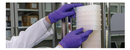
BenchCel's convenient front-loading stacks can be used in a wide variety of environments: benchtop, hood, biosafety cabinet. They accommodate a variety of microplate types including deep well plates.
