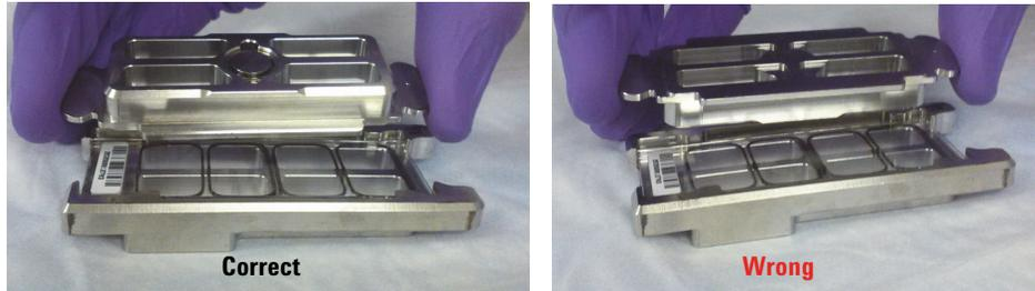
**Figure 9.** Chamber cover in correct (left) and incorrect (right) orientations
