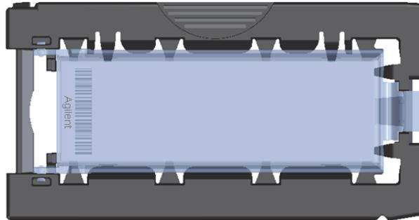
**Figure 21.** Slide inserted in slide holder – cover closed
