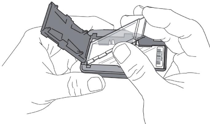
**Figure 22.** Inserting the ozone-barrier slide cover
