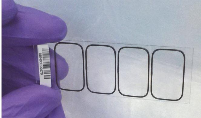
**Figure 4.** Gasket slide, gasket side
