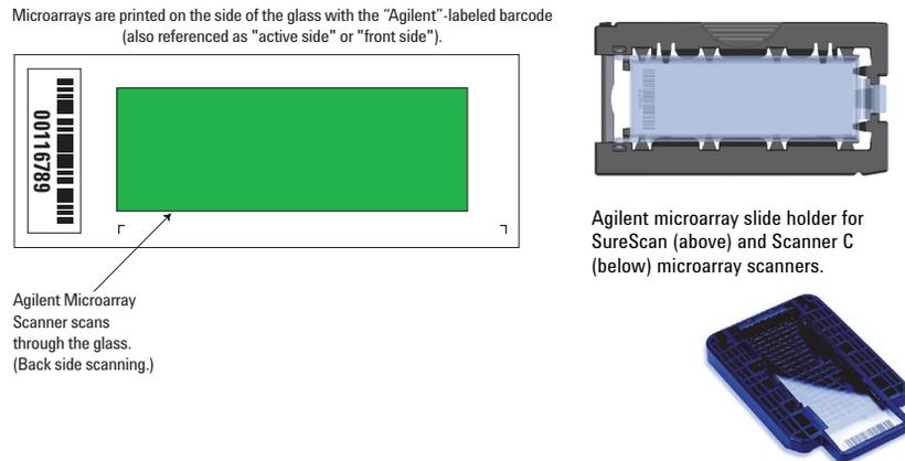
**Figure 31.** Agilent microarray slide and slide holder
