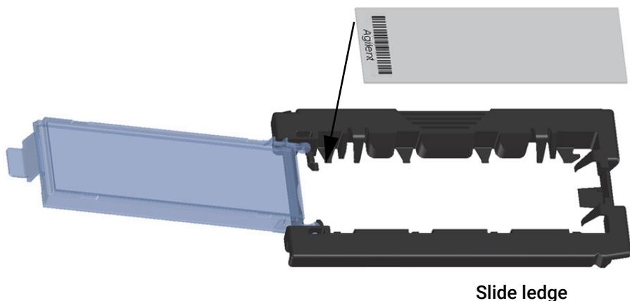
**Figure 19.** Inserting slide into the slide holder
