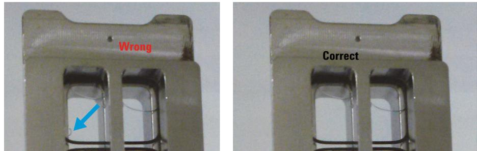
**Figure 13.** The slide on the left shows a stray, stationary bubble (denoted with arrow), which must be removed before hybridization. The slide on the right shows only large mixing bubbles, which move freely around the chamber when rotated. Bubbles are acceptable, as long as they move freely when you rotate the chamber.
