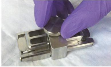
Figure 11. Tightening of the thumbscrew on the clamp
