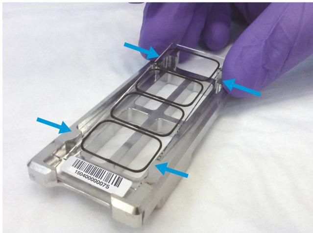
**Figure 5.** Chamber base, guide posts denoted with arrows
