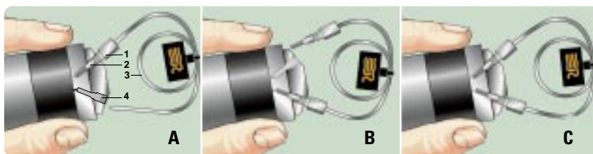
Fig. 6 Cut-away view of stainless steel sample loop installation.
