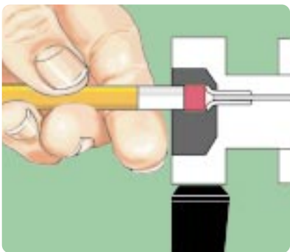
Fig. 1 To reform the needle seal, push the eraser end of a pencil against the needle port.
