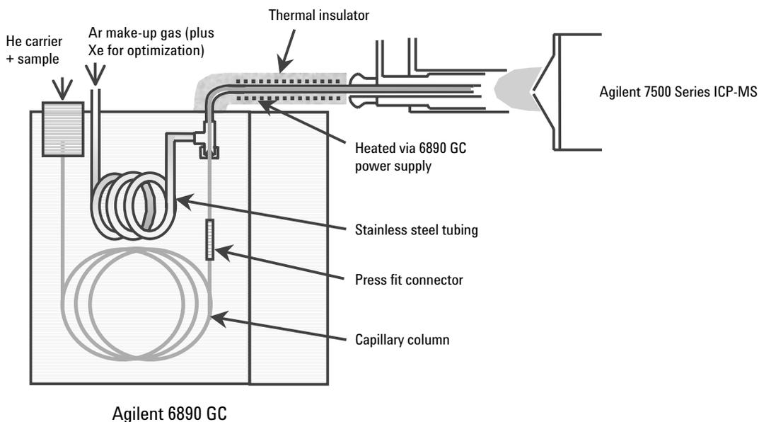
Figure 1: Schematic of GC-ICP-MS interface.
