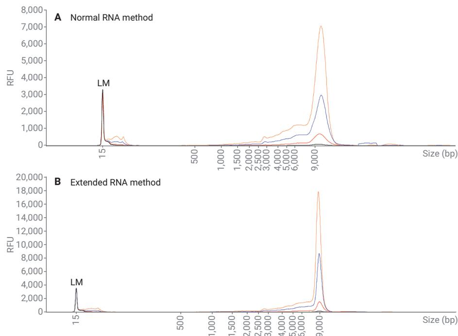
**Figure 2.** Overlay of the 9,000 nt IVT mRNA fragments over a dilution series of 100, 50, 10, 1 ng/μL separated on the Agilent 5200 Fragment Analyzer system with the Agilent RNA kit (15 nt) using the long RNA Ladder and (A) the normal RNA method (B) the extended RNA method. LM = lower marker.
