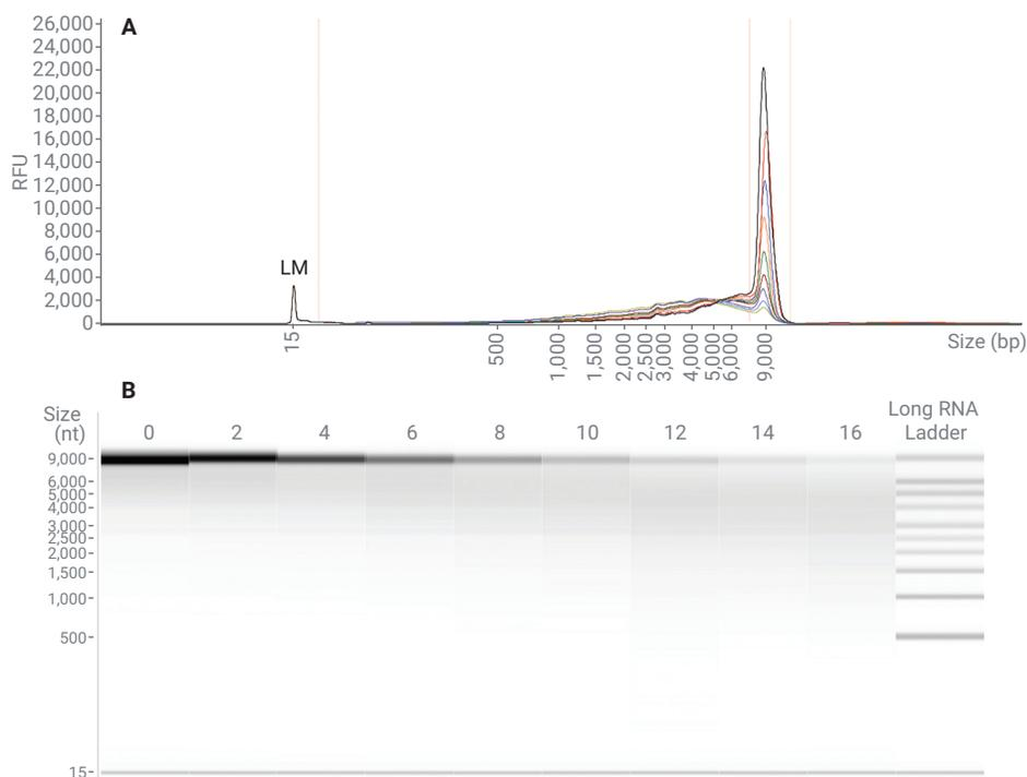
**Figure 4.** 9,000 nt IVT mRNA analyzed on the Agilent 5200 Fragment Analyzer system with the Agilent RNA kit (15 nt) using the long RNA Ladder and extended RNA method over a degradation series at 70 °C from 0 to 16 minutes. (A) Electropherogram overlay of degradation series. (B) Gel image of degradation. LM = lower marker.
