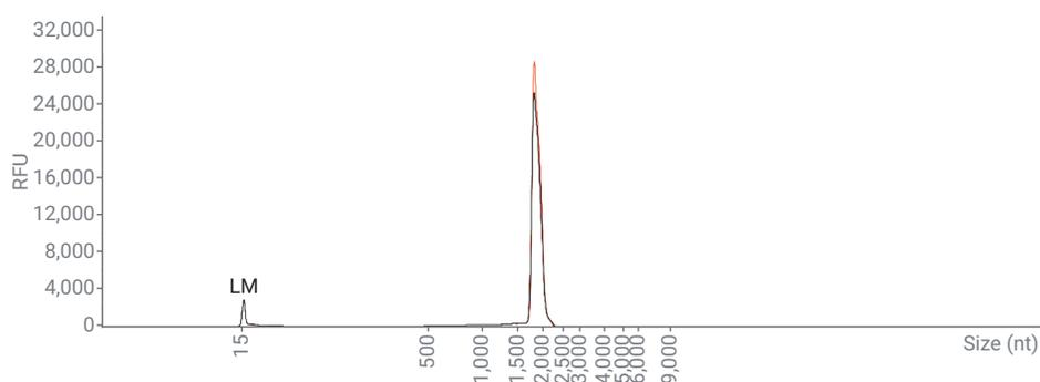
**Figure 5.** Overlay of the 1,800 nt IVT mRNA fragments capped (red) and uncapped (black) separated on the Agilent 5200 Fragment Analyzer system with the Agilent RNA kit (15 nt) using the extended RNA method and the long RNA Ladder. LM= lower marker
