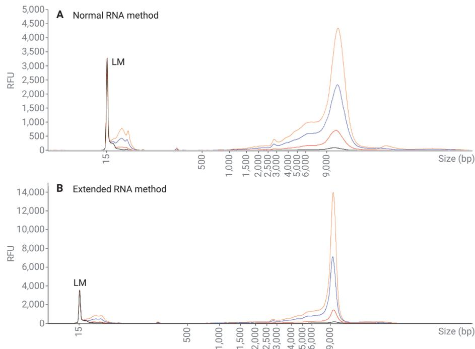
**Figure 3.** Overlay of the 10,000 nt IVT mRNA fragments over a dilution series of 100, 50, 10, 1 ng/μL separated on the Agilent 5200 Fragment Analyzer system with the Agilent RNA kit (15 nt) using the long RNA Ladder and (A) the normal RNA method (B) the extended RNA method. LM = lower marker.
