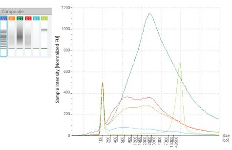
**Figure 2.** Analysis of purified genomic DNA from FFPE samples using the Agilent 4150 TapeStation system with the Agilent Genomic DNA ScreenTape assay and corresponding reagents. The left panel is the gel image, and the right panel is the electropherogram. A1 is the ladder provided along with the gDNA kit (100 bp-48.5 kb), B1-E1 correspond to FFPE samples 1-4, and H1 is the FFPE DNA standard.
