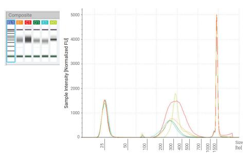
**Figure 3.** Analysis of the precapture libraries obtained with the Agilent 4150 TapeStation system, Agilent D1000 ScreenTape assay, and related reagents. The left panel is the gel image, and the right panel is the electropherogram. The main peak of the library corresponds to the highest point, and is about 300 bp for all samples, with the fragments mainly concentrated within 200-500 bp.
