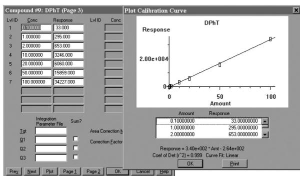
Figure 2: GC-ICP-MS Calibration Table and Calibration Plot.
