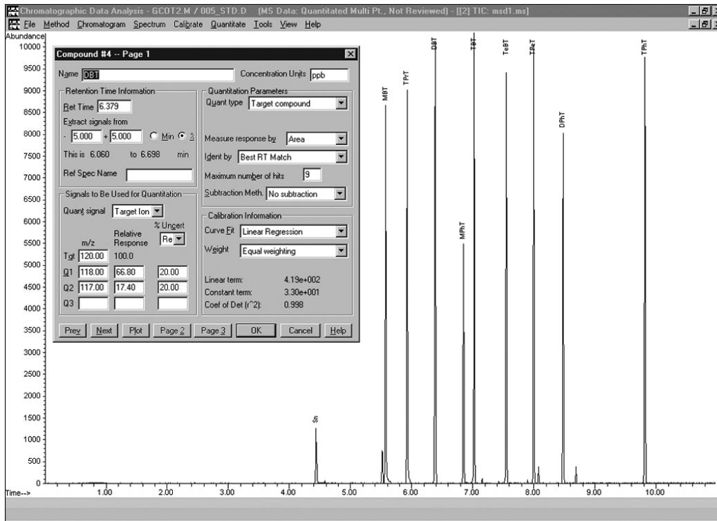
Figure 1: Plasma Chrom software window showing organotin chromatogram by GC-ICP-MS and interactive calibration setup.
