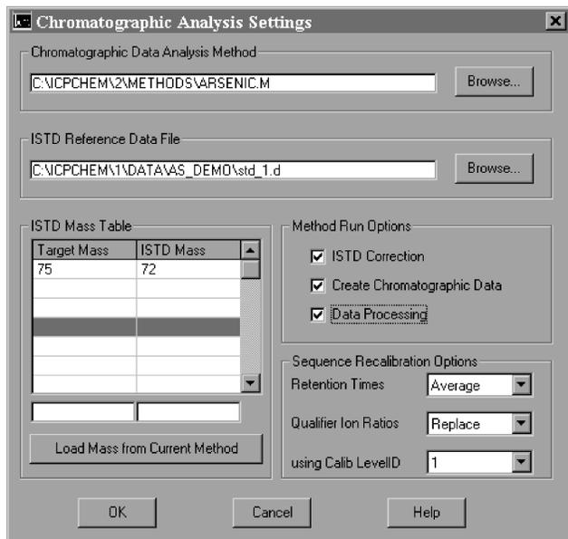
**Figure 4. Chromatographic Settings Window linking Plasma Chrom Data Analysis to ICP-MS Data Acquisition. Note selection of plasma internal standard and sequence recalibration options.**
